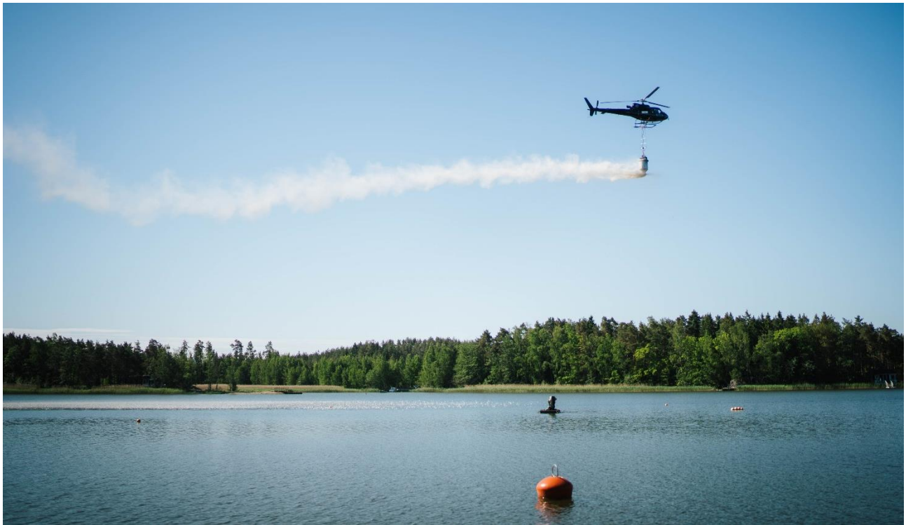
Fig. 3. In SEABASED pilots, activated limestone was spread from a helicopter.
